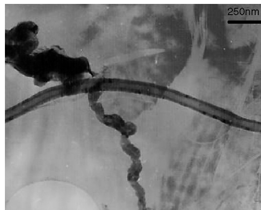
Fig. 2. TEM image of the purified MWNTs.
